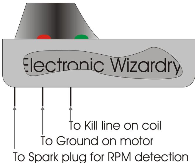
**OFF:** The kill line is closed (shorted) mechanically and power is removed from the auto shutoff circuit.
