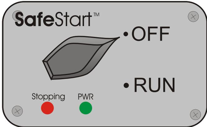
**Stopping:** Lights up when the circuit is commanding a motor kill—possible in the RUN position. If the engine RPM exceeds 3000 RPM within 5 seconds of starting, the kill line is shorted for 5 seconds then the light goes out and the system resets.
